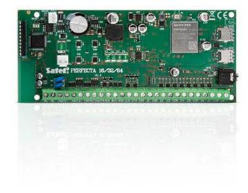
(listening for sounds from the protected premises). The module supports two nano-SIM cards to ensure uninterrupted communication: if transmission over the first operator's network fails, the second card is automatically selected.
